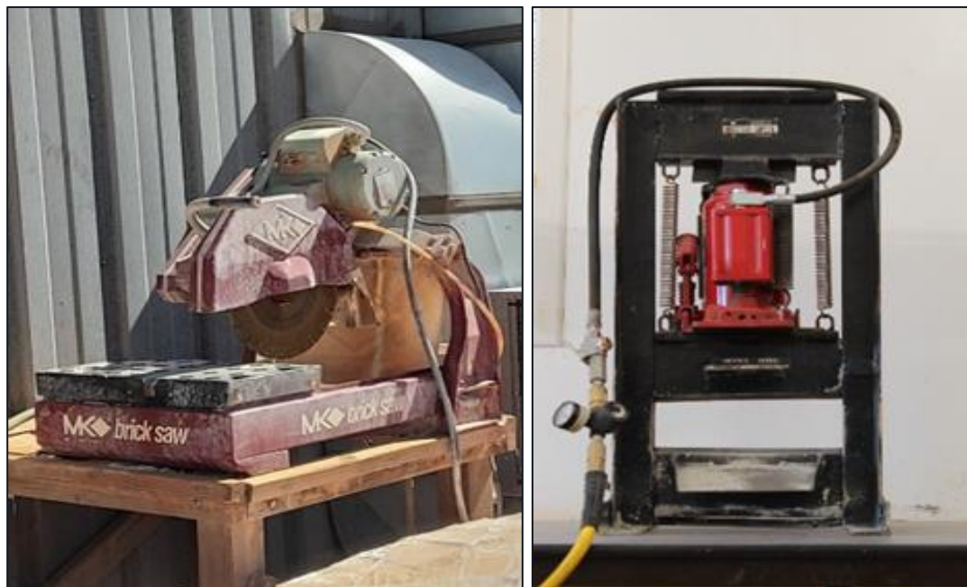
Figure 10-3: Cactus Project's Rock Saw and Hydraulic Splitter
