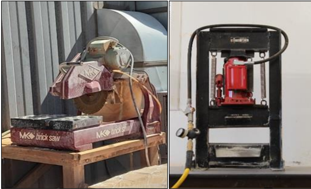
Figure 10-4: Cactus Project's Rock Saw and Hydraulic Splitter
